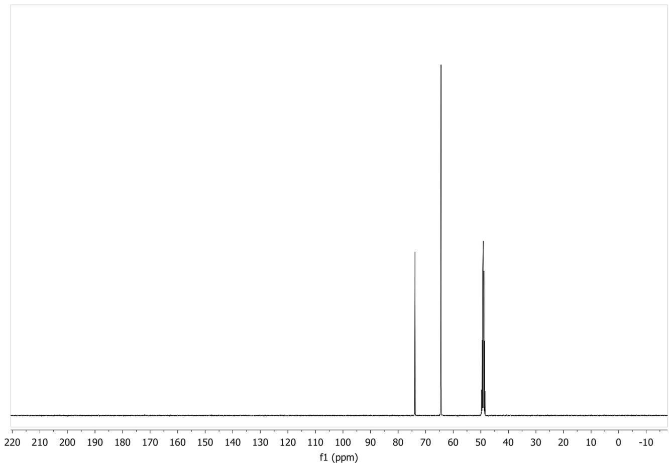
**Fig. 3**  $^{13}\text{C}$ -NMR spectrum of purified glycerol
