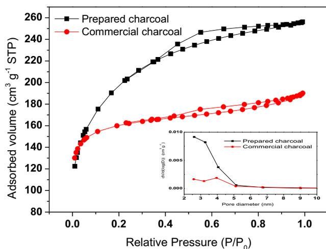
**Fig. 1** Nitrogen adsorption and desorption isotherms of prepared and commercial charcoals
