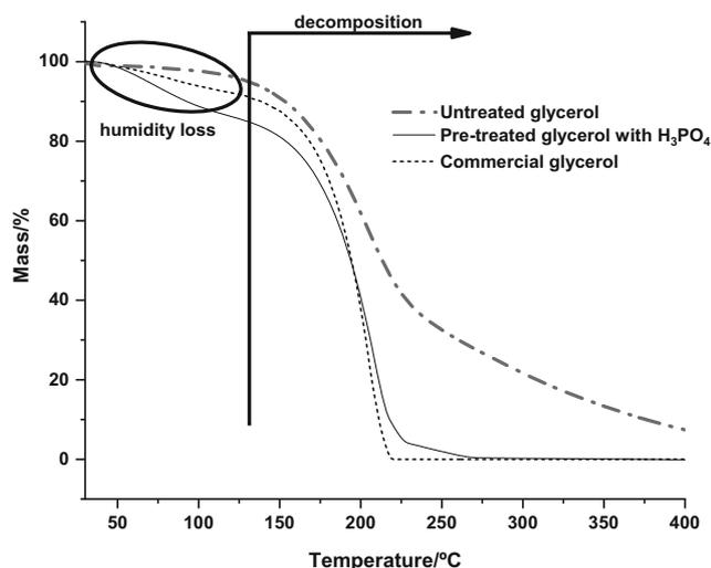
**Fig. 5** TG curves of untreated glycerol (thick solid line), glycerol pretreated with  $\text{H}_3\text{PO}_4$  (thin solid line), and commercial glycerol (dashed line), under dynamic nitrogen atmosphere at  $50 \text{ mL min}^{-1}$  and heating rate of  $10 \text{ }^\circ\text{C min}^{-1}$
