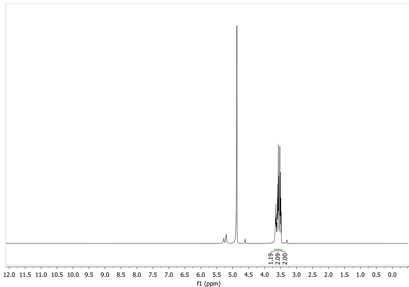
**Fig. 2**  $^1\text{H}$ -NMR spectrum of purified glycerol
