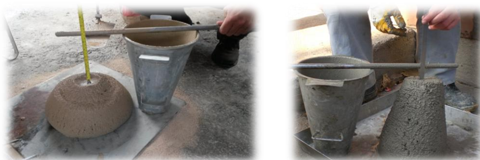
Figura 1 (a) e (b) – Slump Test Argamassa com RCC e Areia Natural.
