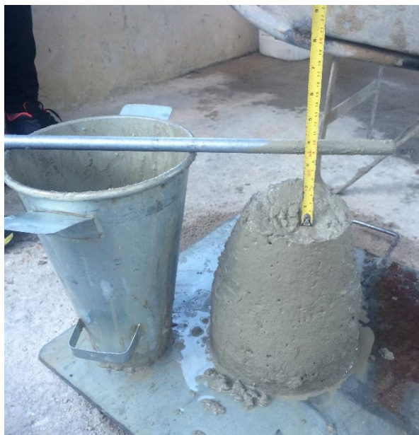
Figura 1 – Slump Test Concreto com areia artificial.
