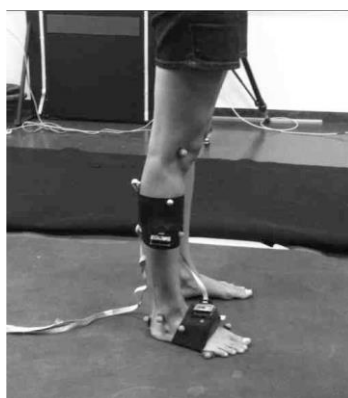
Figure 3 – Positioning of passive markers and accelerometers on the volunteer.
